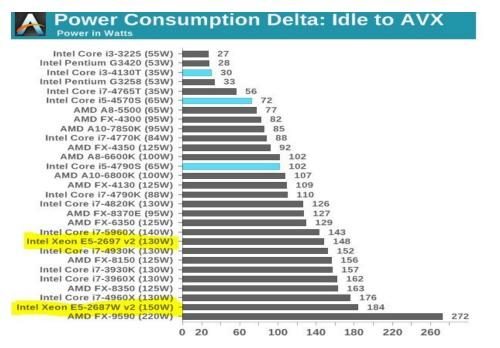
Figure 3.4: Power consumption for two chips of IVYBridge
