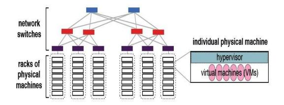
Figure 1.5: Typical data center network
